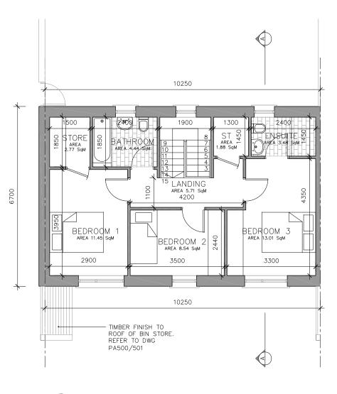
1 PA100/ 1:100 2 PROPOSED FIRST FLOOR PA100 GFA - 58.41SQ M 2 1:100
