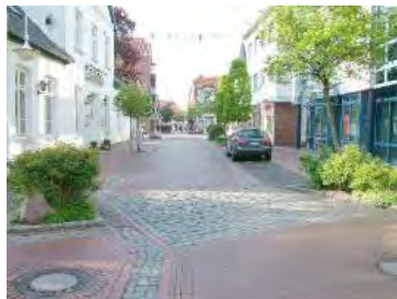
Sample Paving Detail creating Traffic Calming
